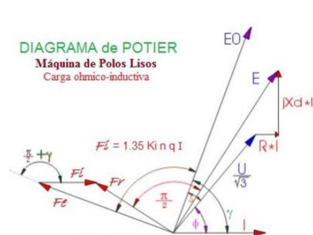
Figura14.- Diag Pottier- Carga RL.
